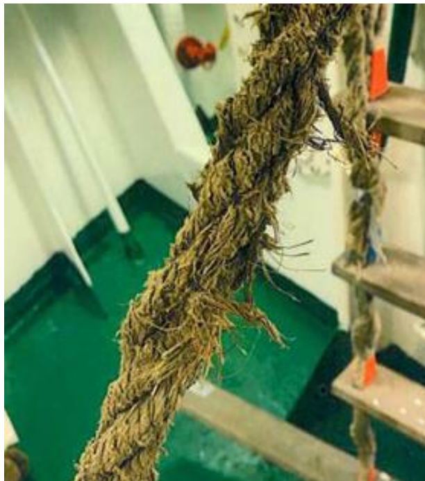
Photo 10: Frayed side rope.
