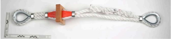
K: 20 mm polypropylene rope, with step and metal clip seizing (sample L the same)
