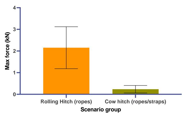
Figure 44: Average max force for rolling hitch compared with cow hitch securing methods.
