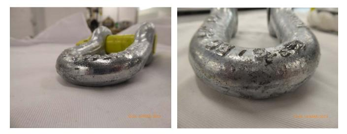
Figure 64 : No visible damage was found on the shackle after any of the tests.
