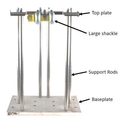
Figure 58: The rig for WP3 D shackle testing with the large shackle arrangement.
