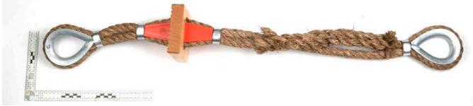
C: 20 mm manila rope, with step and metal clip seizing (sample D the same)
