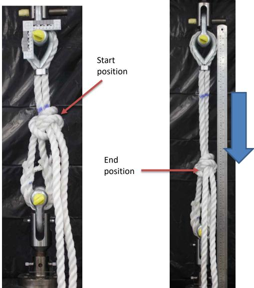
Figure 38: Images showing start and end position of cow hitch S5, that slid 250 mm.
