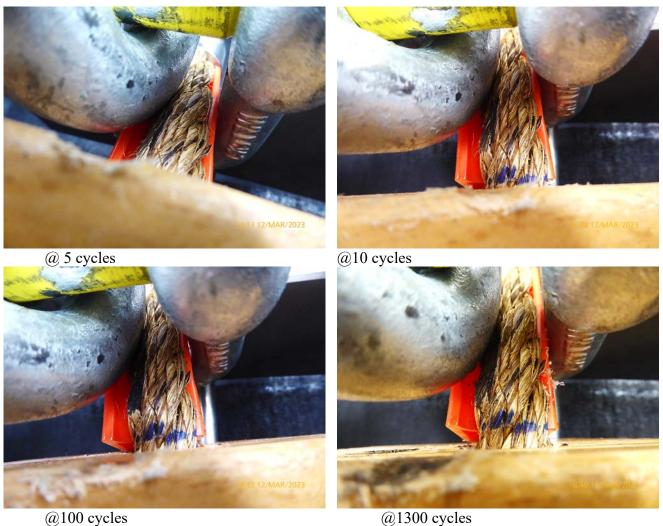
Figure 76 : Specimen G showing the progression of the rope wear during testing for 5 cycles (Top left), 10 cycles (Top right), 100 cycles (Bottom left), and 1300 cycles (Bottom right).
