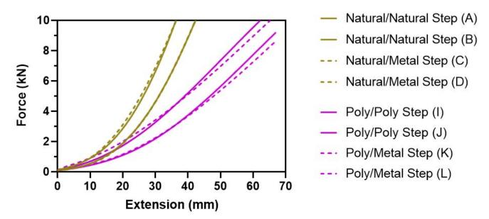
Figure 24: Performance after bedding in stress-strain graph (force-extension) of the behaviour of the Manila and Polyprop ropes with steps under test during run 10.
