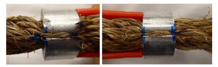
Figure 63 : Specimen H after 1500 cycles showing (Left) permanent plastic deformation to the top of the metal fastener from contact with the small shackle. The top metal fastener slipped 2 – 3 mm from its initial position during the test. (Right) No slippage was observed on the metal fastener underneath the wooden assembly.
