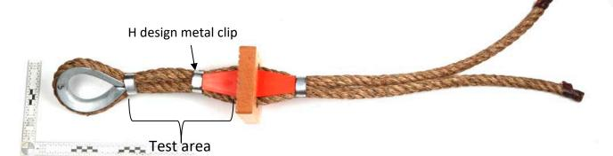
G: 20 mm manila rope, with step and metal clip seizing (sample H the same)
