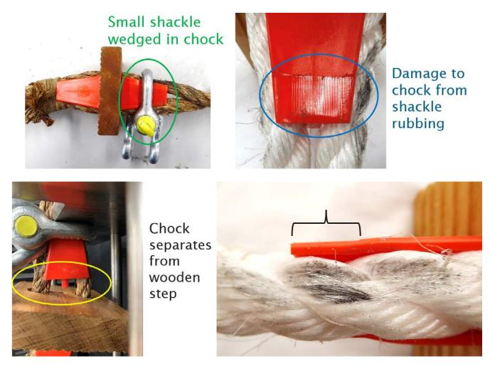
Figure 65 : The small shackle passed over the rope seizing and got wedged in the chock (Top left). When the small shackle was removed after testing, damage to the chock surface was observed (Top Right). The wedging effect resulted in the chock coming away from the wooden step during the 'ladder put away' step (Bottom left). Permanent deformation was observed to the chock (Bottom right).
