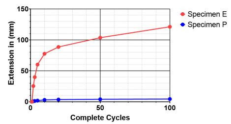
Figure 71 : Specimen E (Small shackle, Manilla, and Rope seizing) extension over 100 cycles with slippage, compared with Specimen P (Small shackle, Polypropylene, and Metal fastener) with no slippage.
