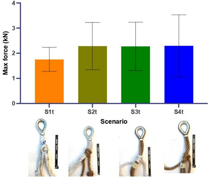
Figure 45: Max force for each rolling hitch scenario.
