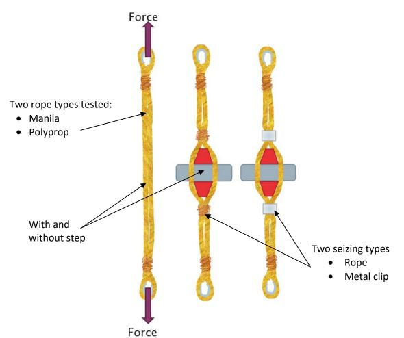
Figure 8: Schematic showing the baseline tensile testing of the rope, the rope with step and rope seizing, and the rope with step and aluminium clip.
