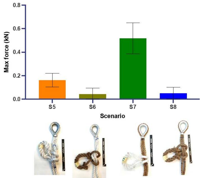
Figure 46: Max force for cow hitch scenarios involving polypropylene and manilla loops.
