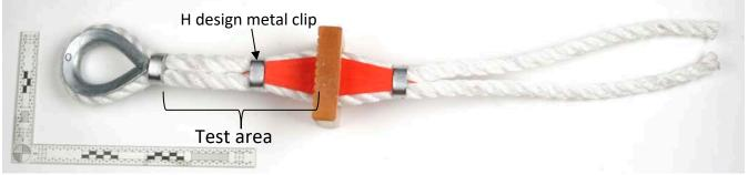
O: 20 mm polypropylene rope, with step and metal clip seizing (sample P the same)
