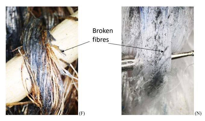
Figure 75 : Macroscope images of the worst worn strands from Manilla and the Polypropylene rope material.
