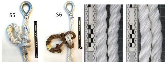
Figure 51: Scenarios 5 and 6 post-test (Left) and the examined worn section of the double rope (Right).
