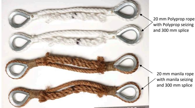
Figure 9: As received condition of samples (no step) for WP1.
