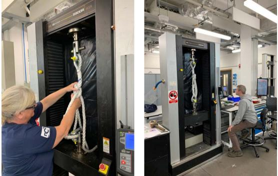
Figure 32: Slip and Grip Scenario 1 being tested on the Instron 6025 electromechanical testing machine.
