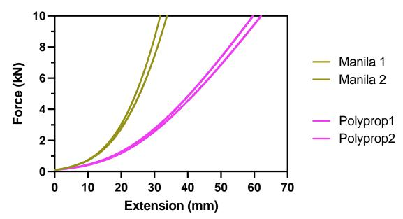
Figure 23: Performance after bedding in stress-strain graph (force-extension) of the behaviour of the Manila and Polyprop ropes without steps under test during run 10.
