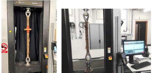
Figure 11: Tested in tension on an Instron 6023 Electromechanical test machine, operating with Instron Bluehill Universal software and fitted with a 100 kN load cell.
