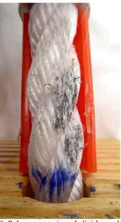
N: Polyprop rope (polyprop seizing) large shackle. O: Polyprop rope (metal clip) large shackle Figure 73 : Specimen F, G, N, and O showing damage to the rope from the large shackle.
