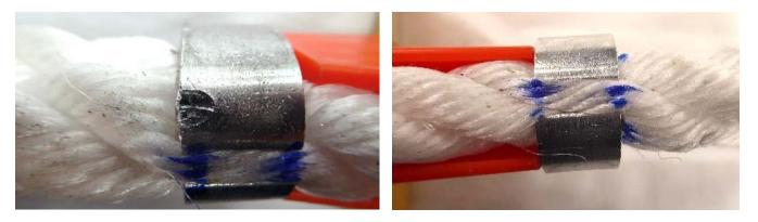
Figure 62 : Specimen O after 1500 cycles showing (Left) permanent damage to the top metal fastener from contact with the small shackle. The metal fastener did not slip during the test. (Right) No slippage was observed on the metal fastener underneath the wooden assembly.
