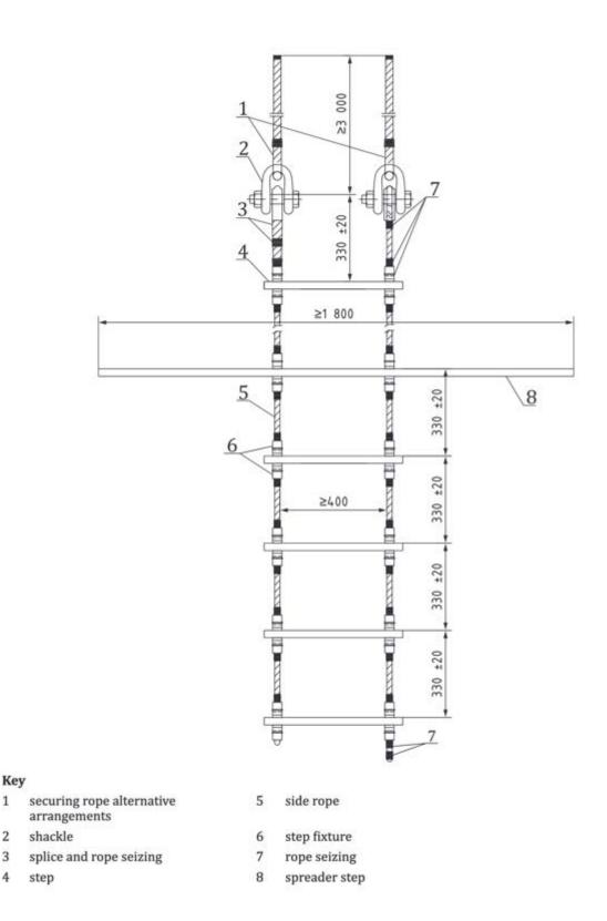
Figure 2: Construction details of a typical pilot ladder from BS ISO 799-1 2019.
