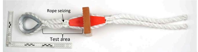
M: 20 mm polypropylene rope, with step and polypropylene rope seizing (sample N the same)
