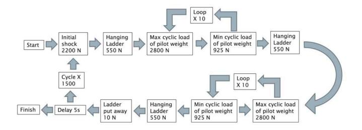
Figure 57 : Schematic showing the loading sequence.
