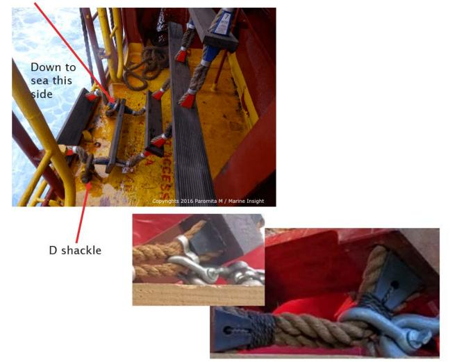
Figure 5: An example of 'D' shackles being used as a tie-off method.
