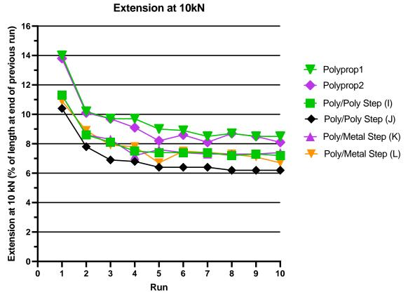
Figure 19: The extension in % with a force of 10 kN applied for the polypropylene ropes with steps.
