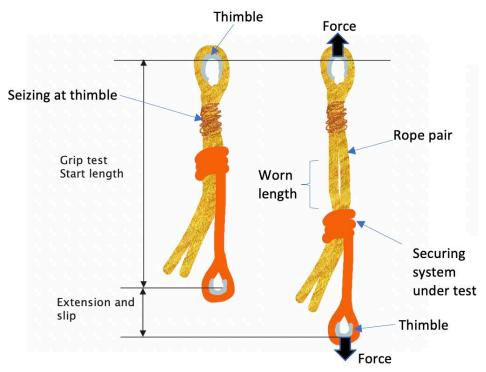
Figure 29: Schematic showing the pre-test arrangement (Left) and the expected post-test arrangement.
