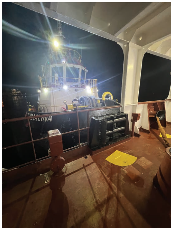
Figure 5: Ship BBC Kimberley , length 139 metres, with pushing tug Turmalina , 72 tons bollard pull. Risk of damaging ship's railing
